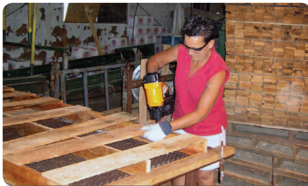
Worktable too high, forcing awkward arm posture.
