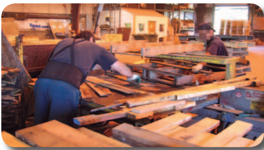
Band saw used for recycling pallets.
