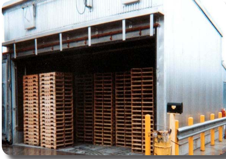
Commercially manufactured heat treatment chamber.
