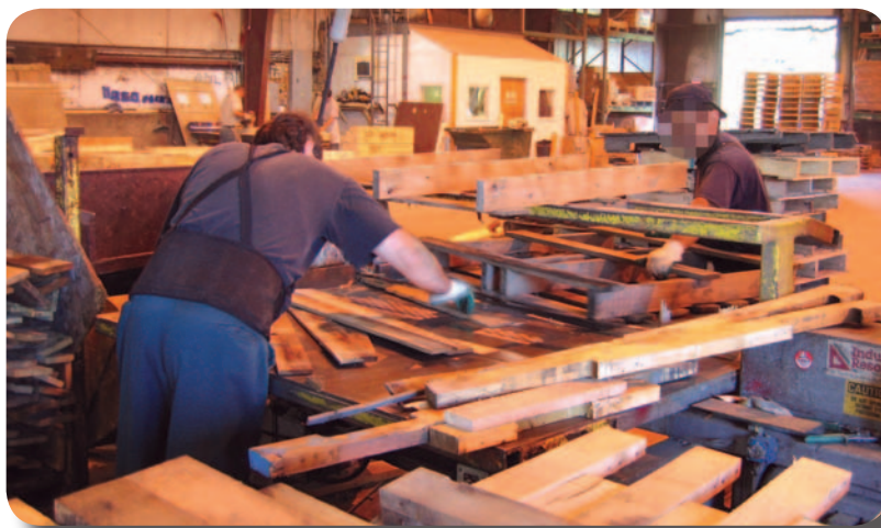
Worker moving pallet through saw.
