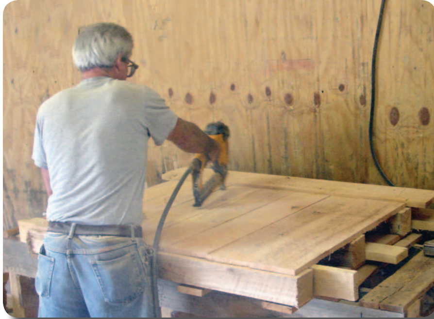
Worker stretching to nail far side of pallet.
