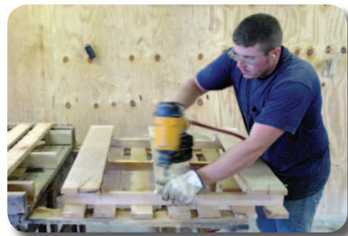
Worker using a nail gun to assemble a pallet.
