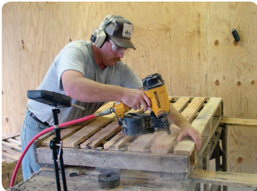
Worker in awkward posture due to table height with work on the far side of pallet.
