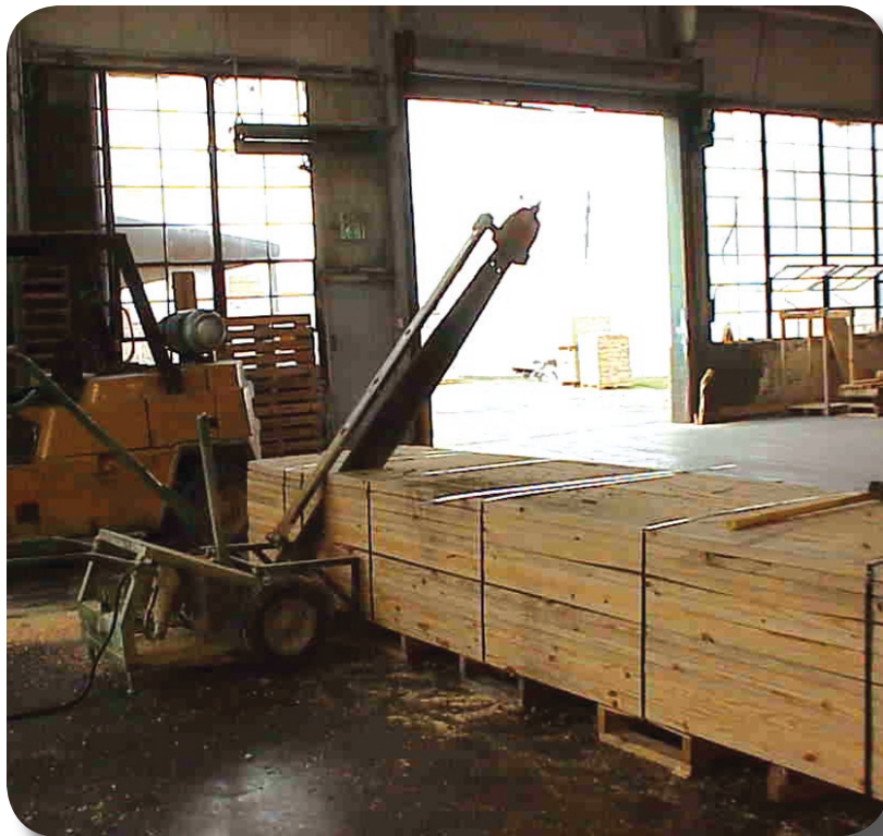
A large chain saw with minimal guarding, no exhaust ventilation, and no barriers to prevent other workers from walking into the saw.
