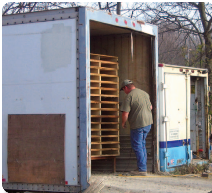
Home-made heat treatment chamber with pallets loaded, and ready to start heat treatment cycle.
