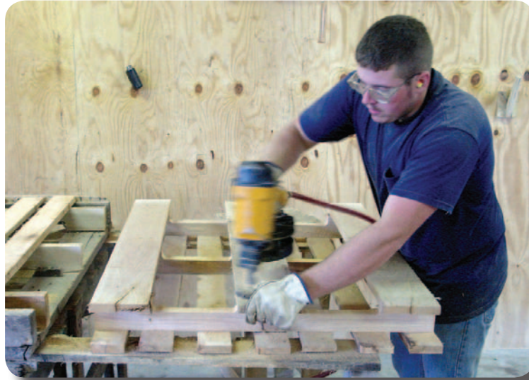
Figure 1. Worker wearing ear plugs to protect against impulsive noise while using a nailgun to assemble a pallet.
