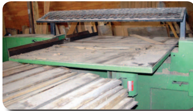
Band saw for recycling pallets that has a guard on top.
