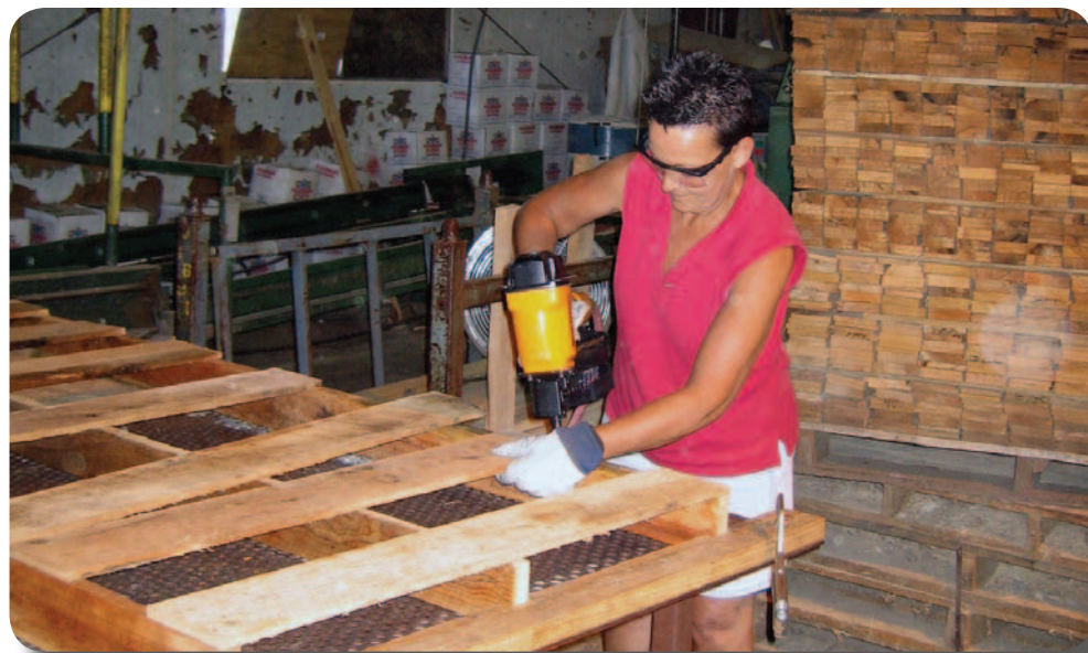
Worktable too high, forcing awkward arm posture.
