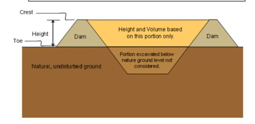
**NOTE:** On slopes, the height of the dam should be measured from the downhill or downstream toe of the dam to the lowest point on the crest of the dam.
