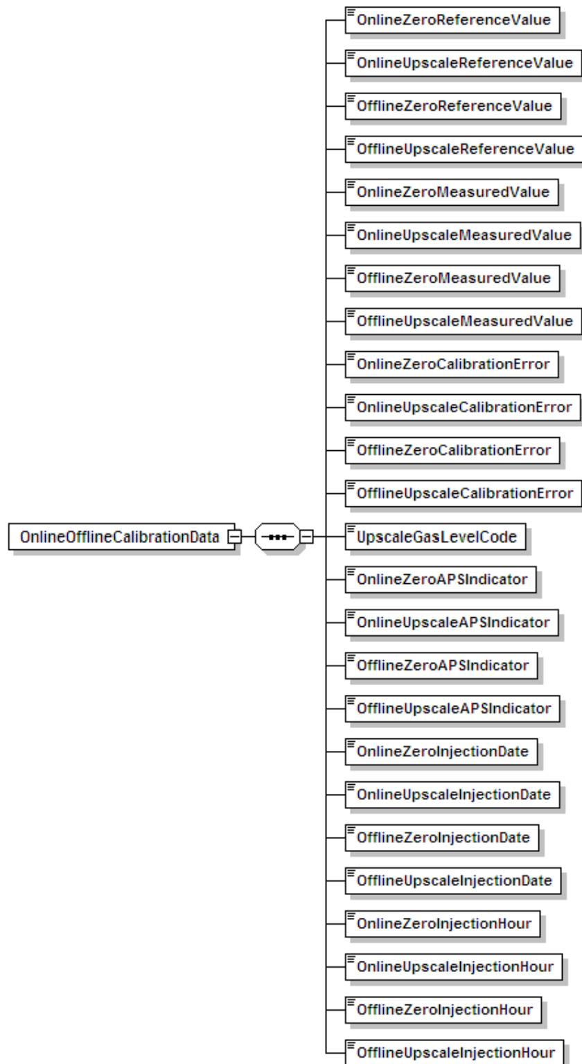
Figure 24 ONLINE OFFLINE CALIBRATION DATA XML Elements
