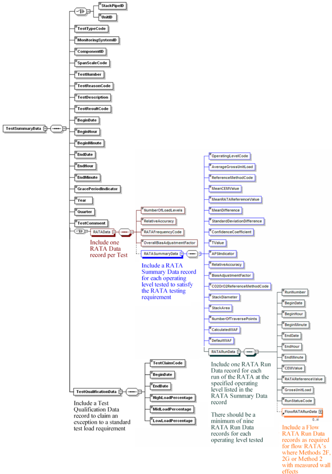
Figure 12a RATA Test XML Structure
