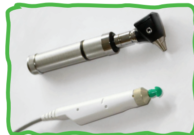
Otoscope (top) and instrument to test how well eardrum moves in response to sound (below)
