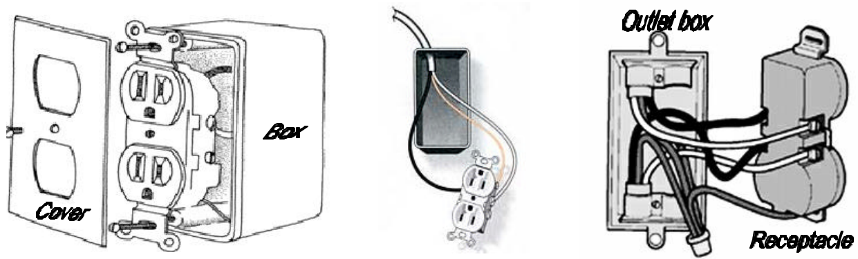
Figure 3 - Outlet Boxes with Installed Grounded Receptacle
