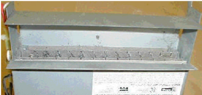
Photograph 2: Close up view of the heating element on the incident heater.
