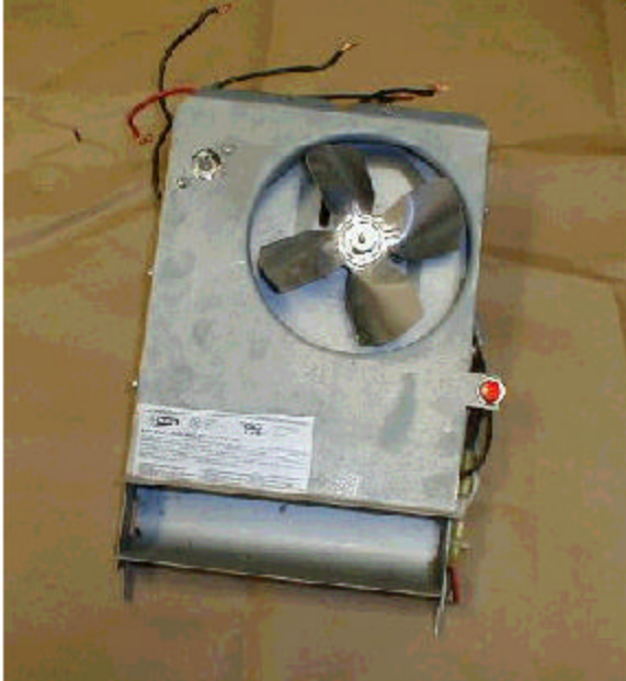
Photograph 1: Photograph shows a front view of the electric forced air heater involved in this IDI.
