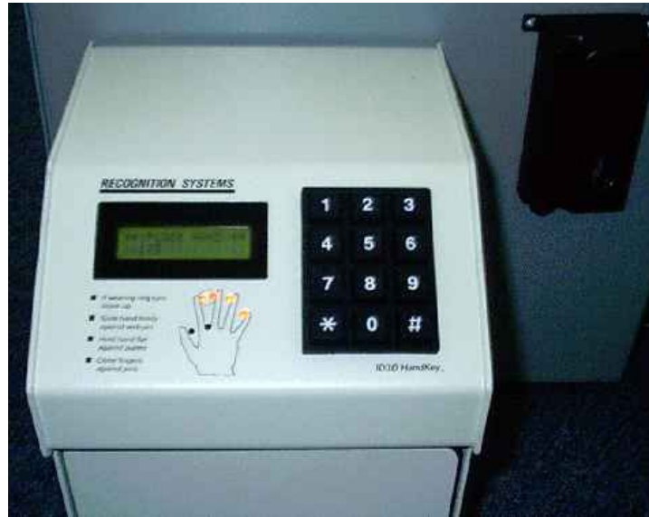
Figure 4. Access Control Reader: Placing Fingers Against Alignment Pins
