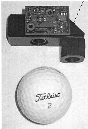
Personal MicroPEM™ optical bench shown with golf ball to illustrate overall size of prototype
