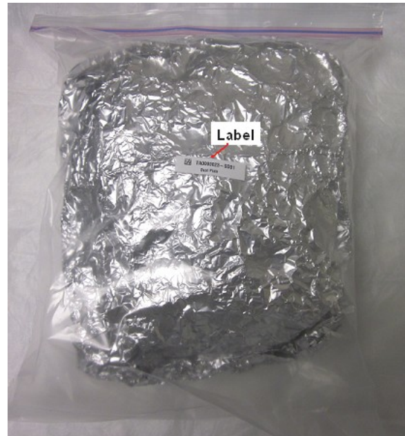
Photo 4. VBD sample: vacuum bag wrapped in aluminum foil, placed in sealed resealable plastic bag, and the sample ID label affixed on the bag.
