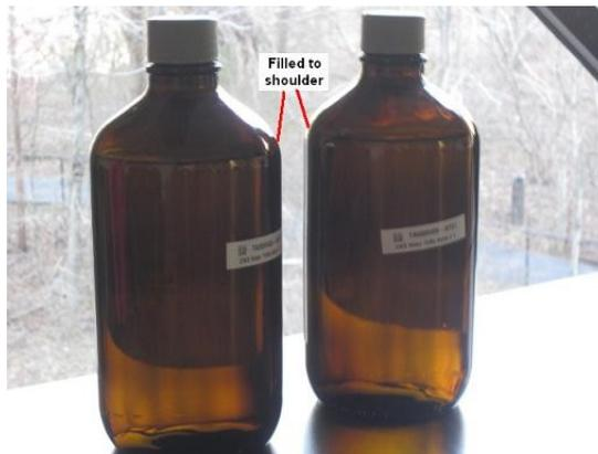
Photo 4. Two bottles filled to the shoulder with water, labeled with sample ID labels.
