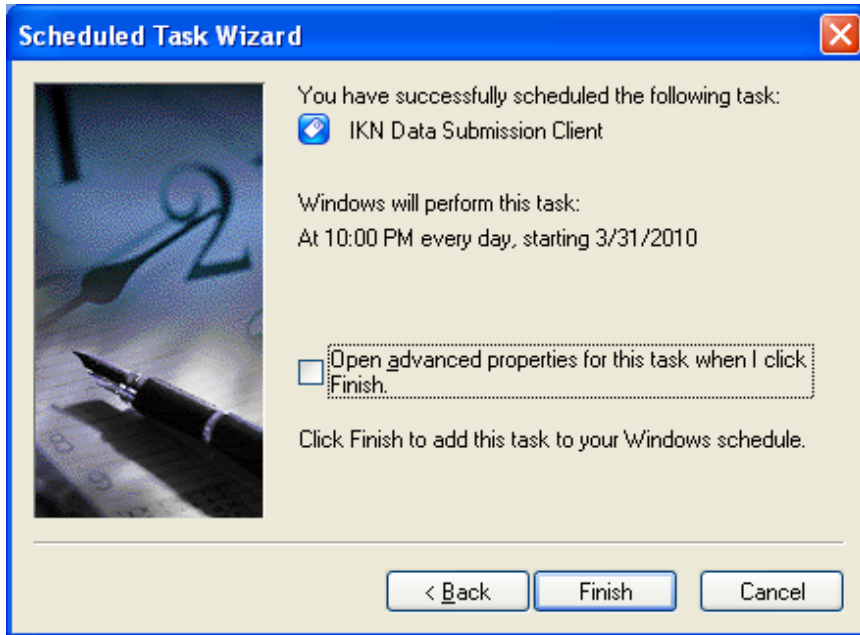
Figure 13: Completing the basic task definition. Click the checkbox to set the advanced properties of the task.
