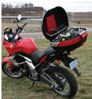
Figure 1. Main DAS unit – carry-over components.
