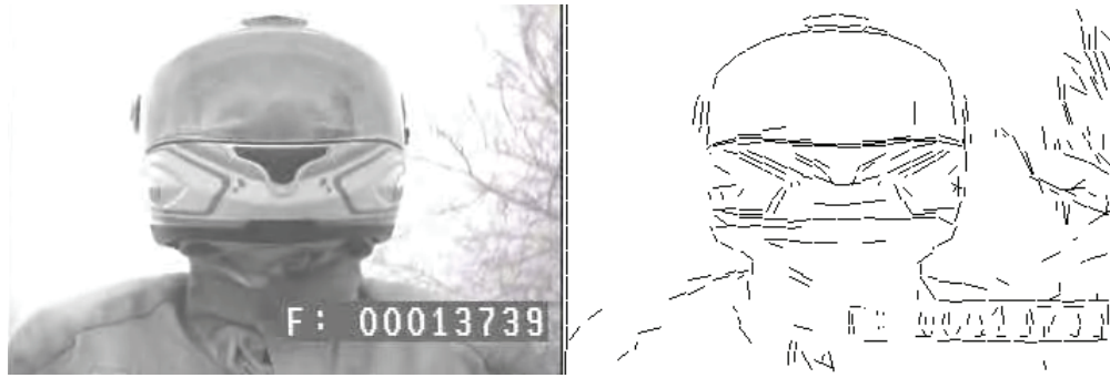
Figure 29. Example one of the pre-processing filters used by the Mask applied to a motorcycle rider.
