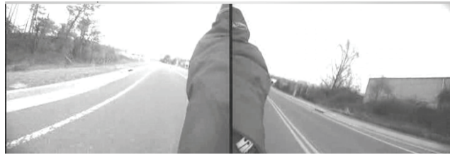
Figure 7. Side-view camera Configuration #2 with mirror-mounted cameras facing rearward.
