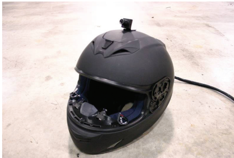
Figure 23. Prototype helmet-mounted eye-tracking system.
