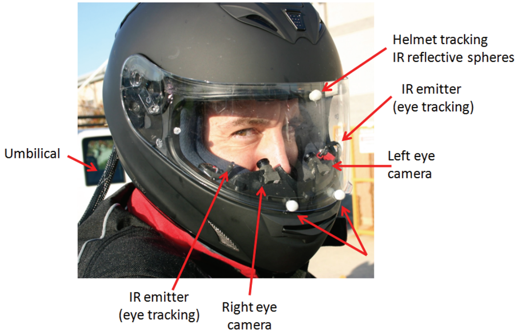
Figure 26. Helmet-mounted eye-tracking system and reflective markers.
