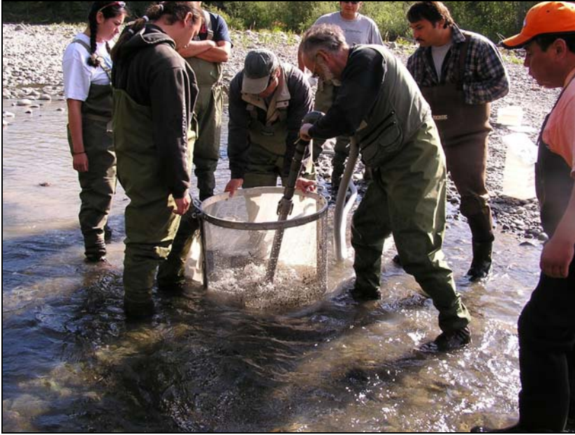
Figure 7. Redds being pumped. A pump discharge wand is inserted into the gravel egg pocket. An hydraulic discharge gently forces eggs and fry upwards from the egg pocket into the capture net.
