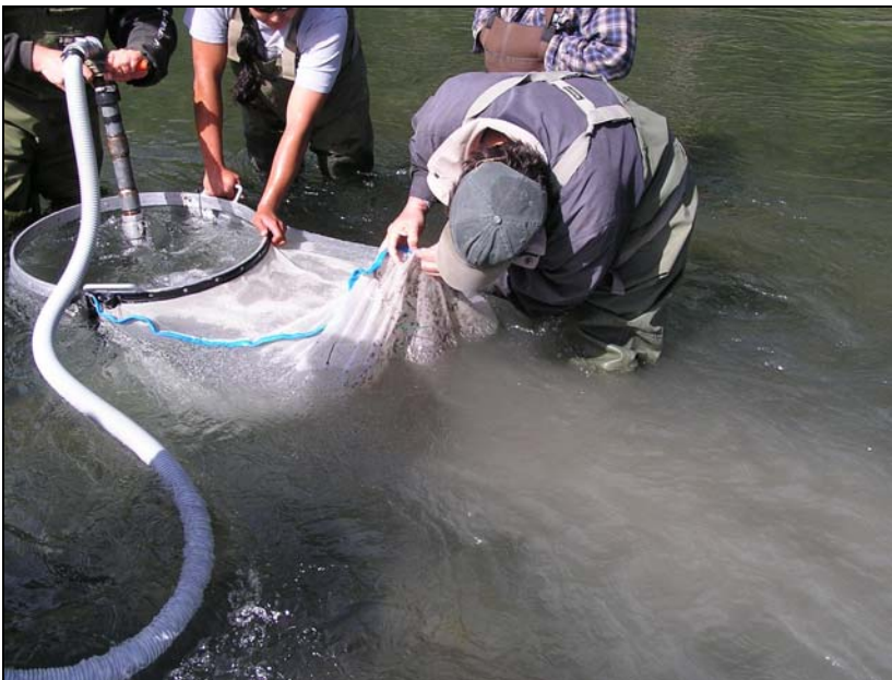
Figure 8. Eggs and fry evacuated from the redd collect in the downstream portions of the capture net. The turbid downstream discharge from the pump site leaves the redd site free for capture of eggs and fry.
