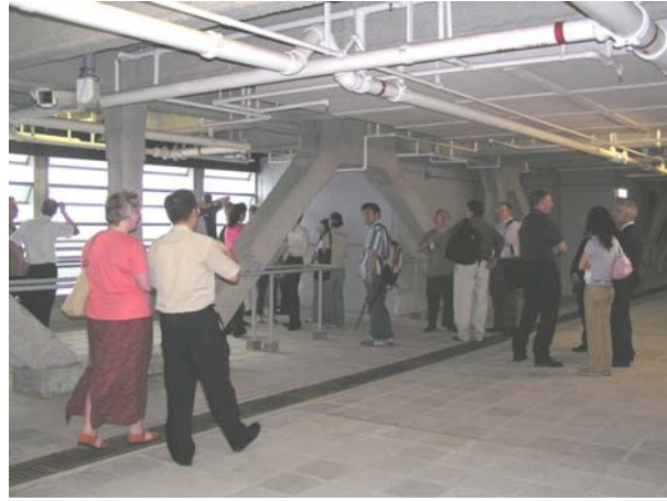
Figure 5 - Refuge floor in a Hong Kong high-rise during a fire drill Source: Arup (used with permission)
