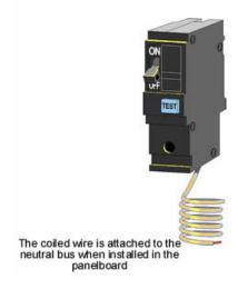
♦ **GFCI Circuit Breaker:** This specialty breaker monitors the circuit for ground faults and opens the circuit when one is found. It also operates as a standard breaker and comes in
