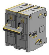
♦ **Duplex Circuit Breaker:** This type of breaker fits on one space or stab in the panelboard and operates two 120-volt circuits. The NEC limits the number of poles allowed in a panelboard to 42. Certain panelboards are classified as circuit limiting. This
