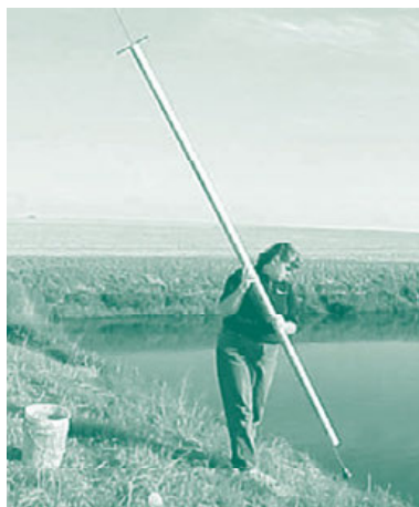
Figure 2. Sampling earthen basin with sampling probe.
