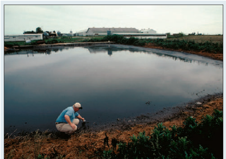
Sampling of wastewater from a lagoon on a hog farm. (Photo courtesy of USDA/NRCS)
