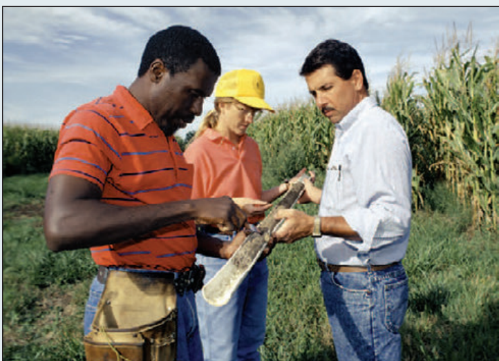
Soil sampling - collection of a soil core. (Photo courtesy of USDA/MO NRCS)
