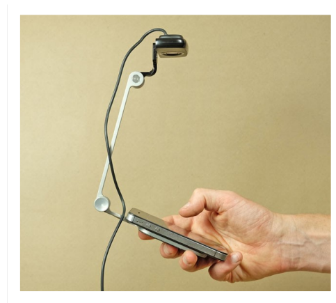
Figure 2: Mr. Tappy Mobile Device Recording Sled 2
