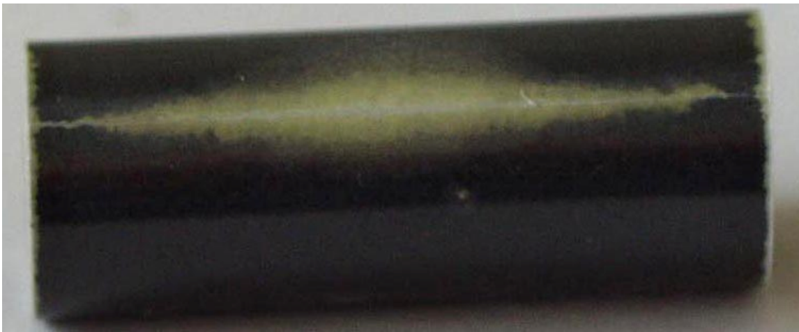
Figure D-5. Outer surface of scratched ZIRLO™ sample following oxidation at 985 °C for 3,400 s. Local hydrogen pickup under the yellow surface was 440 wppm; average pickup was 175 wppm.
