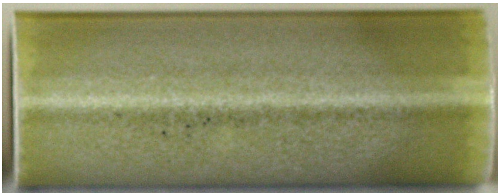
(c) 5,000 s at 1,000 °C; 1,350-wppm hydrogen pickup
