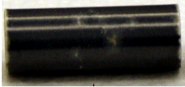
Figure D-7. Outer-surface appearance for ZIRLO™ sample oxidized at 1,000 °C for 4,000 s. Hydrogen pickup was 120 \pm 110 wppm with >280 wppm under the yellow spots.
