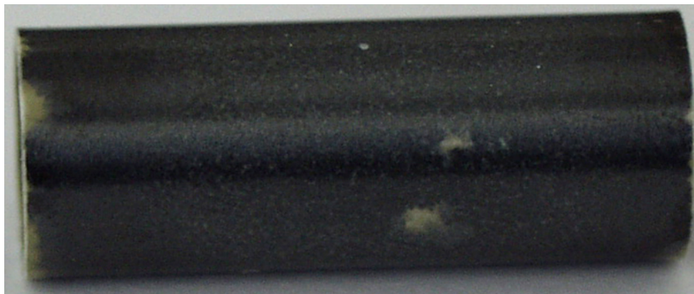
(b) 3,600 s at 1,000 °C; 60-wppm hydrogen pickup
