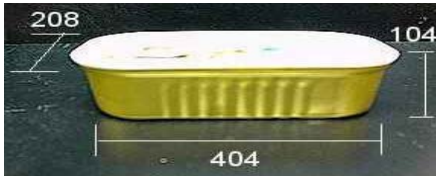
Figure 18 – Measurement of a Low-Profile Container
