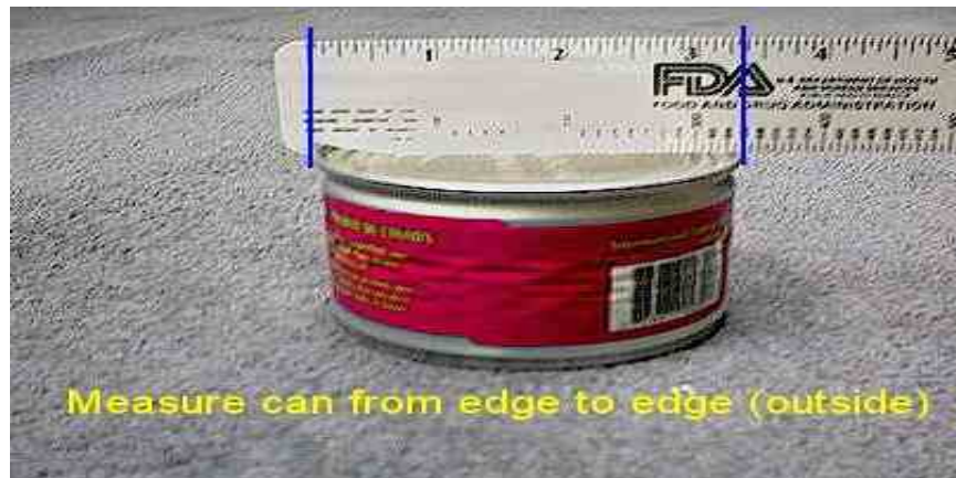
Figure 15 – Measurement of Outer Edges of Container
