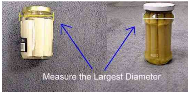
Figure 13 – Measurement of an Unusual Shape Cylindrical Container.
