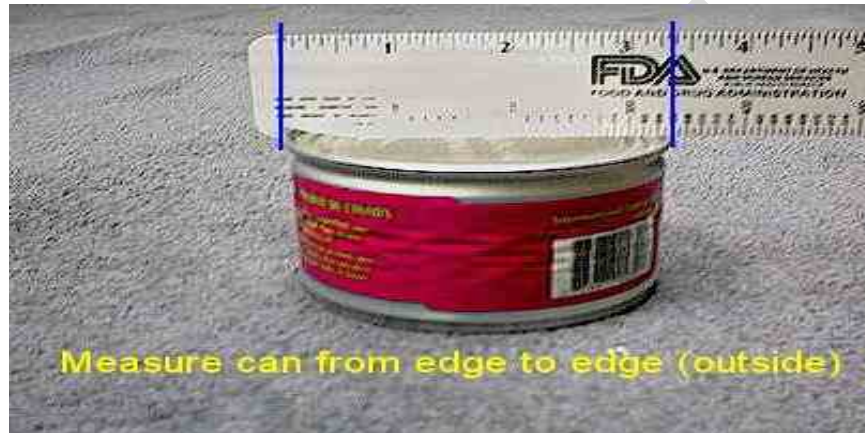
Figure 15 – Measurement of Outer Edges of Container
