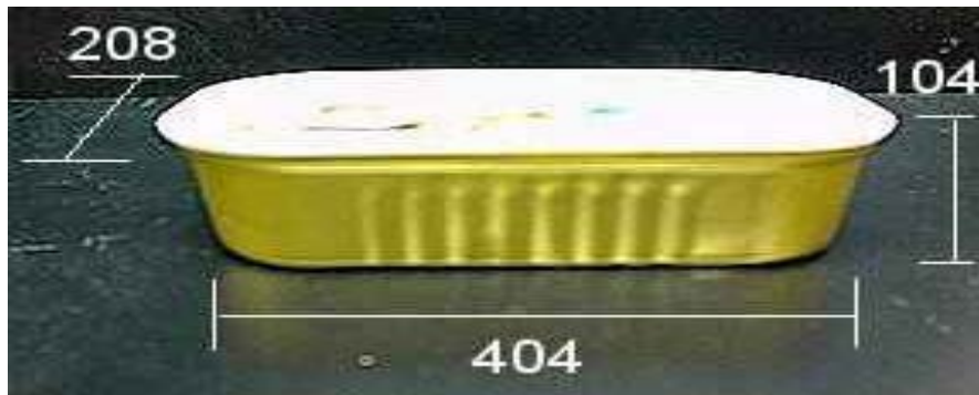
Figure 18 – Measurement of a Low-Profile Container
