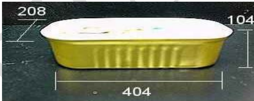
Figure 21 – Measurement of a Low Profile Container
