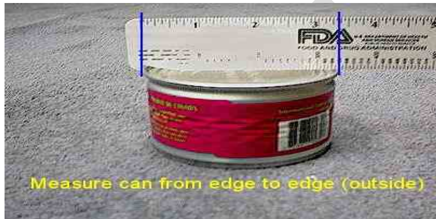
Figure 18 – Measurement of Outer Edges of Container
