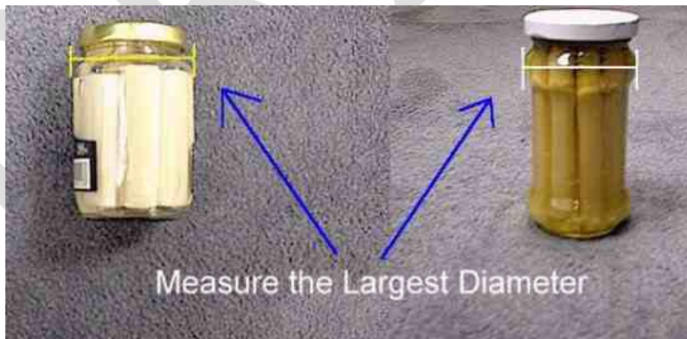
Figure 16 – Measurement of an Unusual Shape Cylindrical Container.
