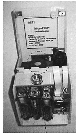
Personal MicroPEM™ showing AA batteries, coin-cell memory battery; and Teflo filter/holder installed in outlet
