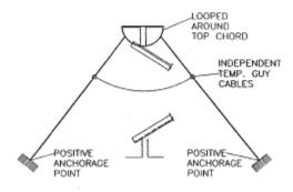
HORIZONTAL BRIDGING TERMINUS POINT SECURED BY TEMP. GUY CABLES DIAGONAL BRIDGING TERMINUS POINT SECURED BY TEMP. GUY CABLES
