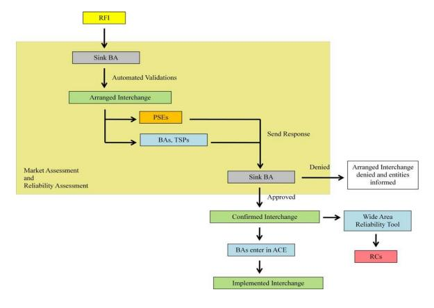
Area Control Error or "ACE" is the instantaneous difference between a Balancing Authority's net actual and scheduled interchange, taking into account the effects of Frequency Bias and correction for meter error.
