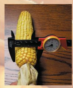
The ear is completely husked so it does not interfere with the caliper jaws. Measurement is taken one inch from the butt of the ear. The ear is in the mouth of the caliper with the jaws at a 90 degree angle to the ear. The caliper is read by reading the top of the caliper to get the tens place, and reading the dial to get the units and tenths decimal. This caliper measurement would be recorded as 46.8mm (add arrows and numbers to show where the 4, 6 and 8 are read if possible)
