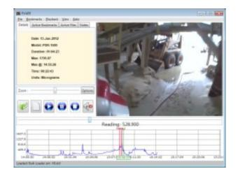
Figure 2. Integrated visual display of worker tasks recorded by Helmet-CAM (top right) and the graph of the worker's dust exposure measured by the aerosol monitor (bottom). The top left shows the EVADE software menu.
