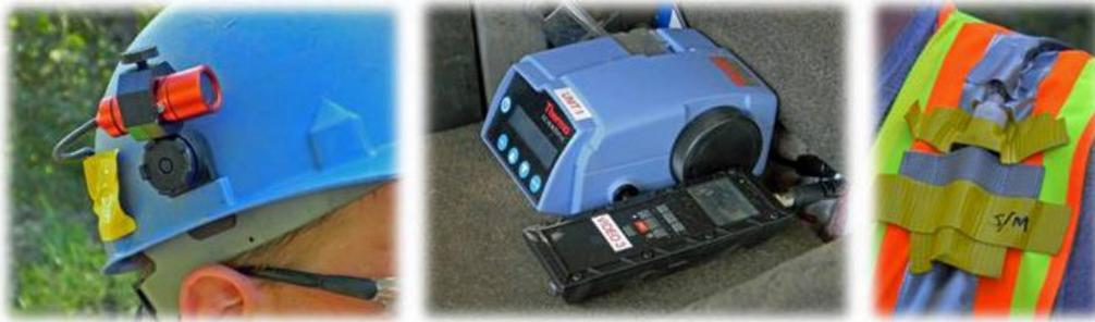
Figure 1. Helmet-CAM system: video camera attached to worker's helmet, pDR-1500 dust monitor and video monitor, and safety vest to hold dust cyclone (shown) and monitors.
