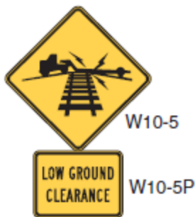
Figure 2-57: Sample Low Ground Clearance Warning Sign
