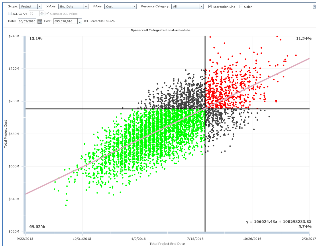
Figure 5.2.8-3 Time-Cost Scatter Diagram: Each data point represents one realization of the simulation
