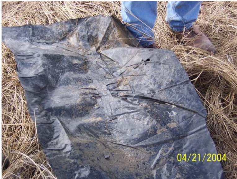
Figure 3.—PE encasement with numerous perforations.
