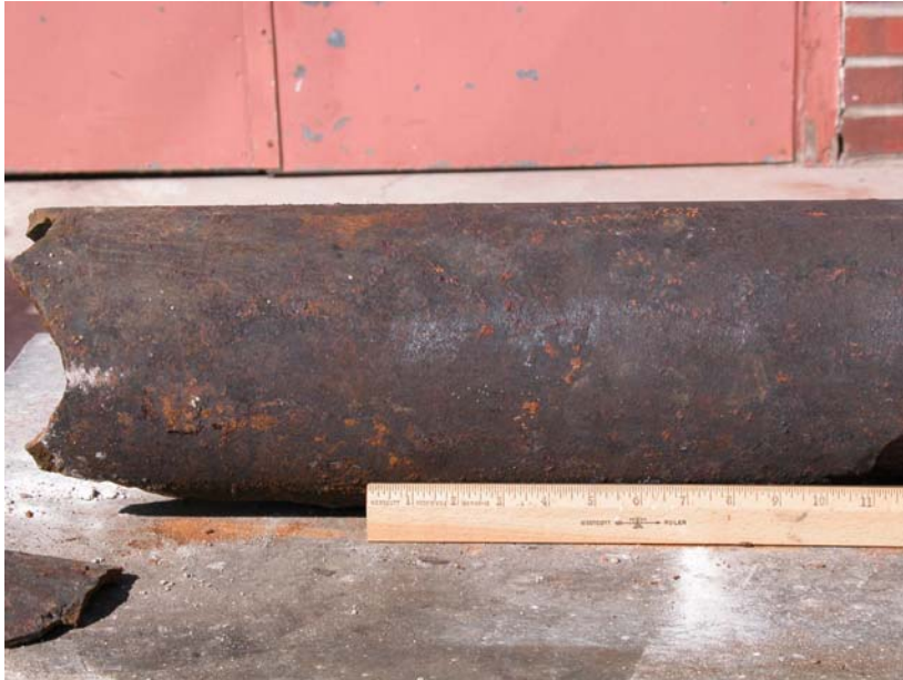
Figure 1: Cast iron pipe section prior to sand blasting. Note color and appearance of surface.
