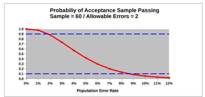
Note: Probabilities are based on the binomial distribution. It is assumed that the sampling fractions are small and that differences from the probabilities for a hypergeometric distribution, which assumes sampling from a finite population without replacement, are minor.
