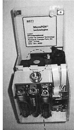
Personal MicroPEM™ showing AA batteries, coin-cell memory battery; and Teflon filter/holder installed in outlet
