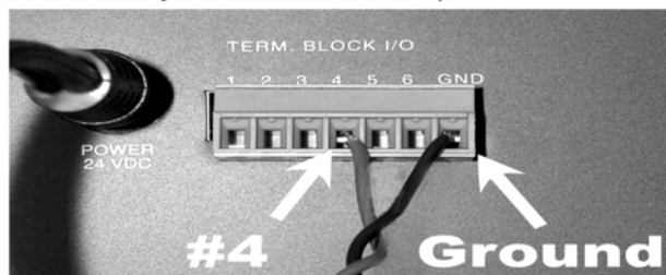
Detail of Terminal Block I/O located on back of the Rheodyne® EV750-100 6-port valve.
