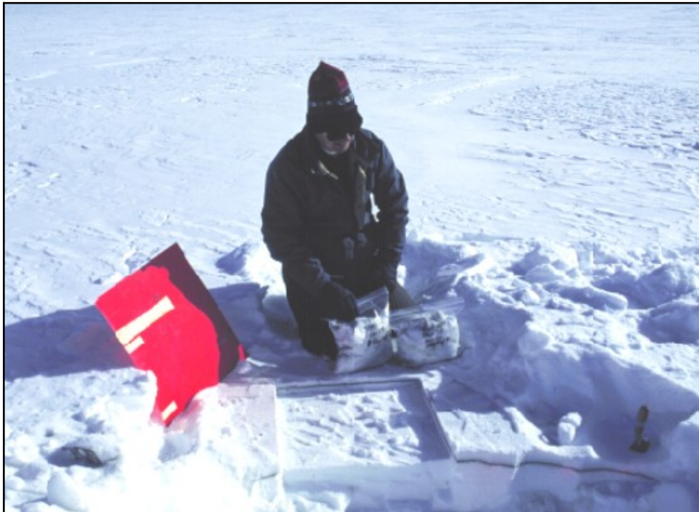
Figure 1. Collection of measured-area ash samples from snow pack after the 1992 eruption of Crater Peak/ Mount Spurr, AK (photo taken on 9/24/92).
