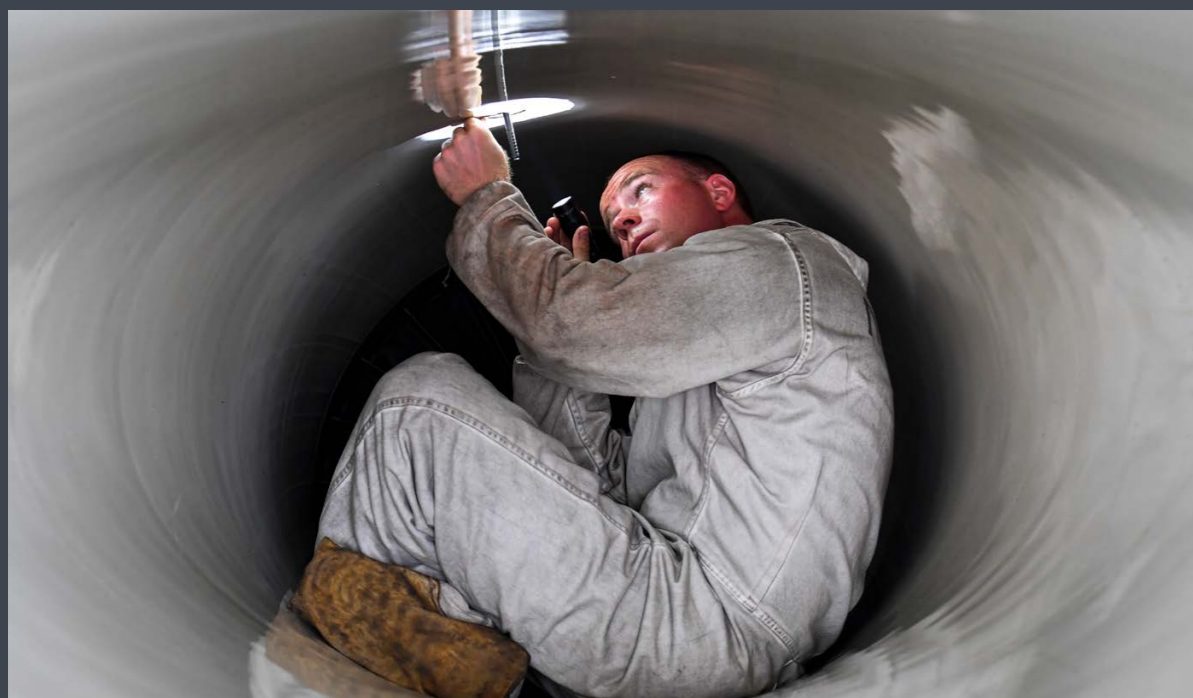
U.S. Air Force Staff Sgt. Todd Hughes checks the anti-ice detector during an intake inspection on a Thunderbirds F-16C Fighting Falcon aircraft at Daytona Beach, Fla., Feb. 24, 2017. The Thunderbirds performed a flyover during the opening ceremonies of the Daytona 500 race Feb. 26. Hughes is a dedicated crew chief assigned to the team. (U.S. Air Force photo by Tech. Sgt. Christopher Boitz)
