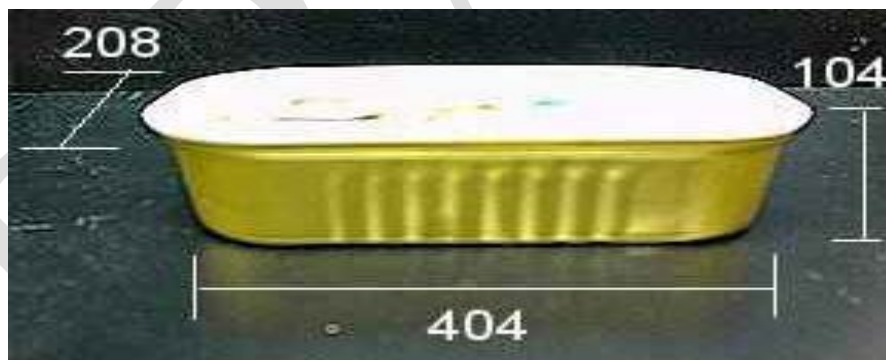
Figure 18 – Measurement of a Low-Profile Container
