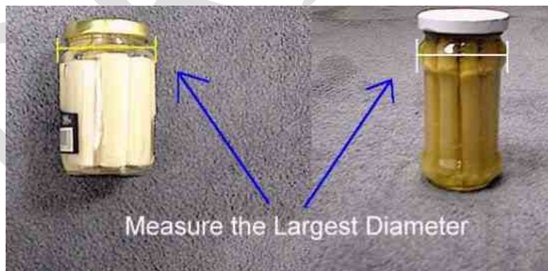
Figure 13 – Measurement of an Unusual Shape Cylindrical Container.
