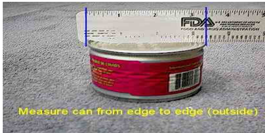
Figure 15 – Measurement of Outer Edges of Container
