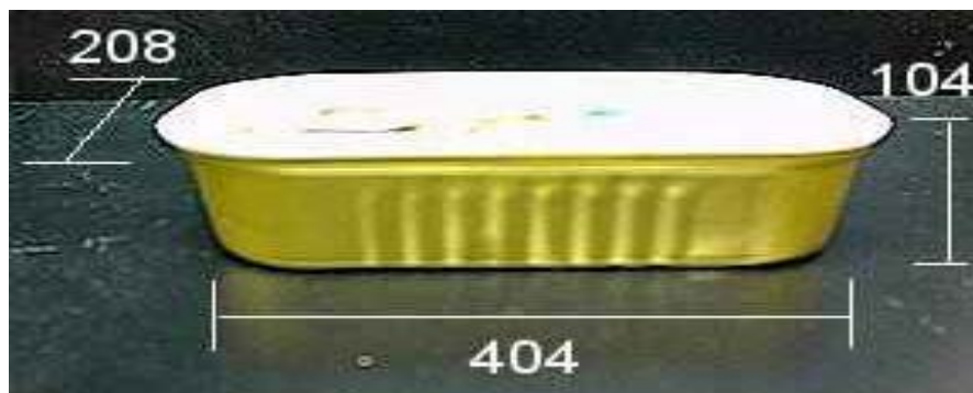
Figure 18 – Measurement of a Low-Profile Container
