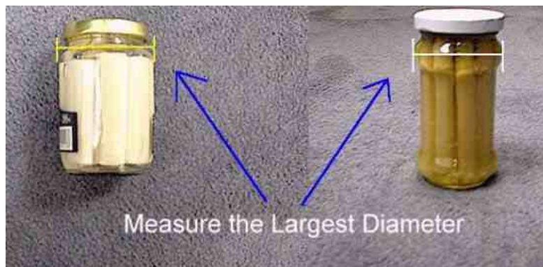
Figure 13 – Measurement of an Unusual Shape Cylindrical Container.
