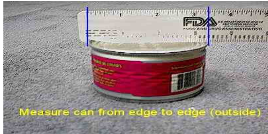
Figure 15 – Measurement of Outer Edges of Container
