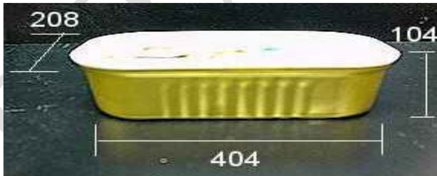
Figure 18 – Measurement of a Low-Profile Container
