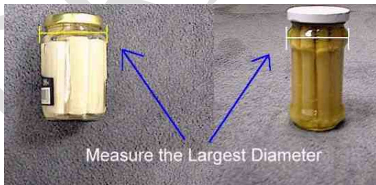
Figure 13 – Measurement of an Unusual Shape Cylindrical Container.
