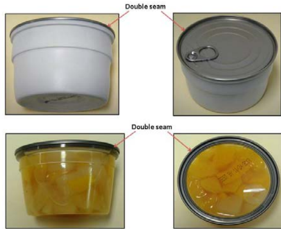
Figure 9 – Semi Rigid Body with an Aluminum Double Seam
