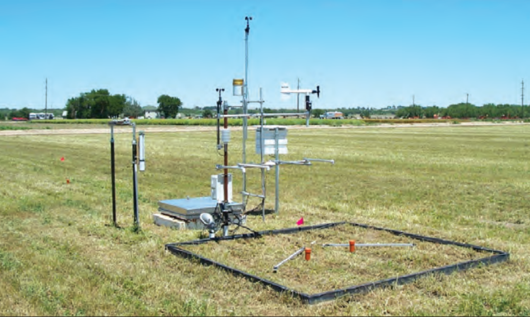
Figure 2. A view at the Arkansas Valley Research Center of the large lysimeter and associated sensors.
