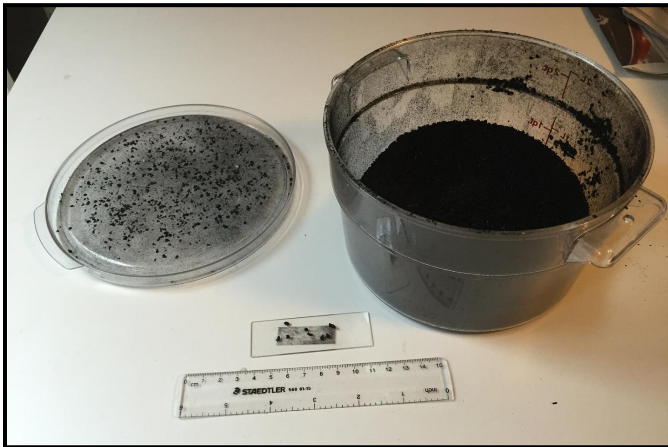
Tire crumb sample in container with lid, calibration slide, and ruler (6 inch / 15 cm).
