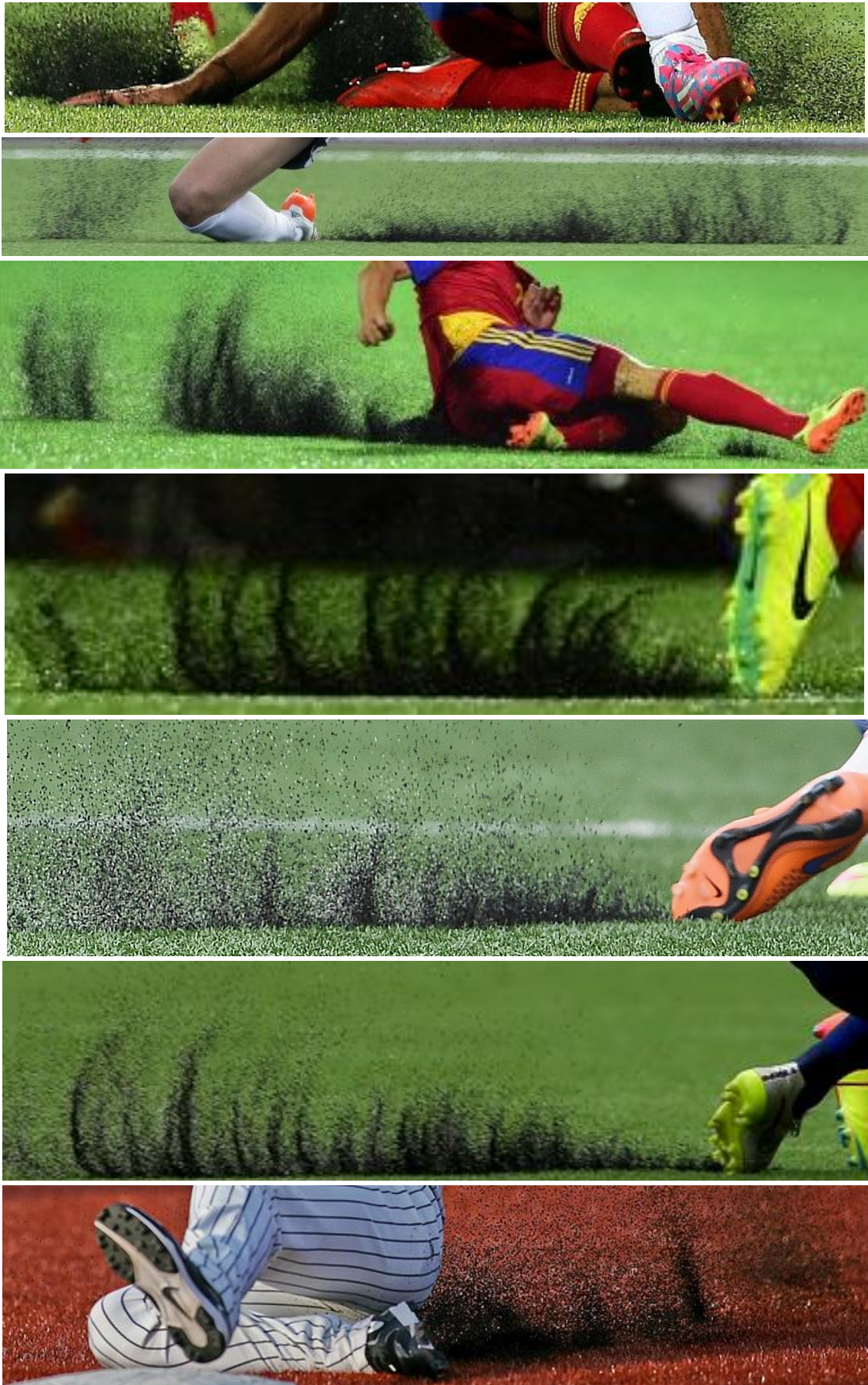
... the on the field activity acts as a mortar and pestle to further break down the tire crumb into dust.
