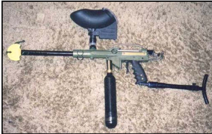
Figure 2: Paintball Marker with a Vertical Bottle Attachment
