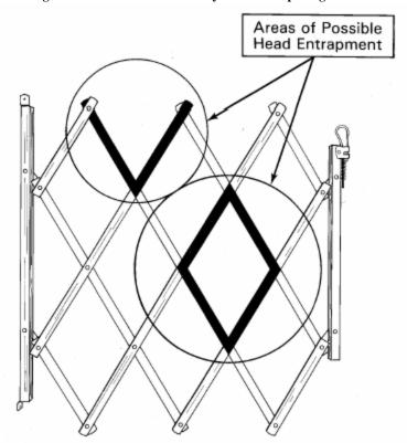
Figure 1: Bounded and Partially-Bounded Openings
