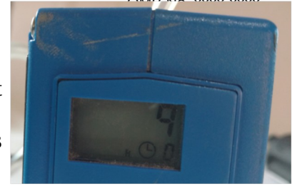
Figure T1-4. Pump window showing elapsed time in minutes (9 minutes in this figure).
