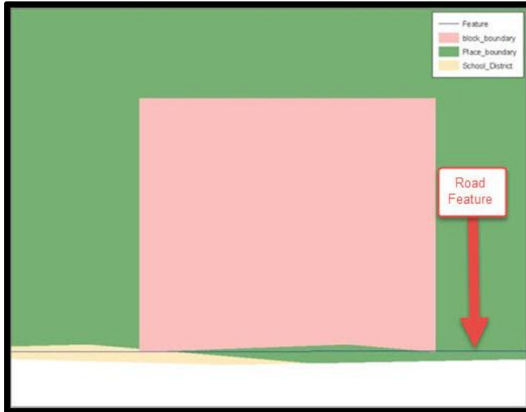
Example 3: This example shows an overlay of four different feature classes. Notice how the topological relationship is compromised. The block, place, and school district boundaries, which are supposed to follow the road feature, are no longer aligned with the road in several locations.
