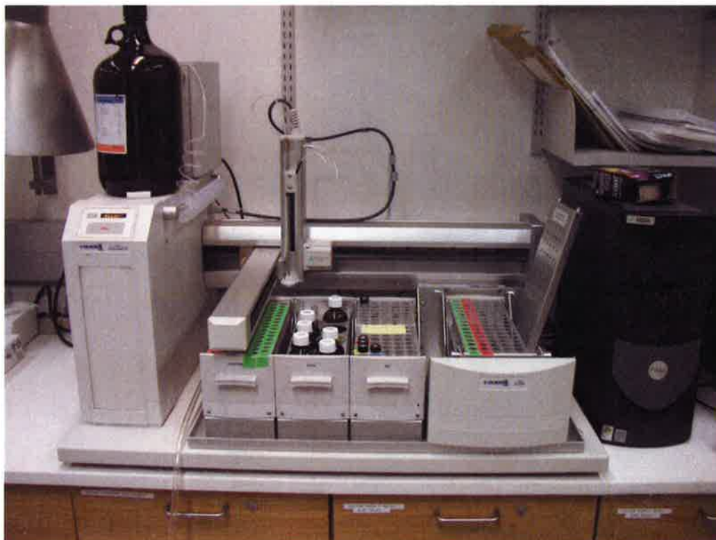
Figure 1. Gilson 215 Liquid Handler used for automated additions of internal surrogate standards and water to the serum samples with mixing by rotation in-between the additions. This equipment also adds recovery standard to GC vials.
