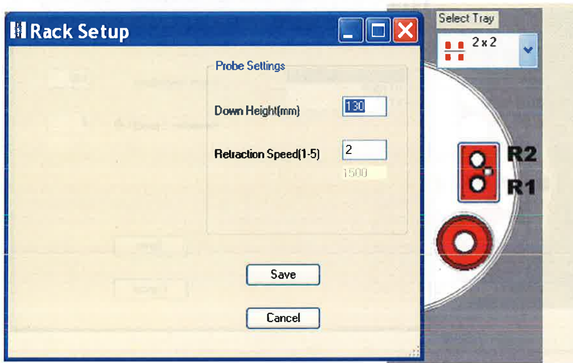
Figure 3d. ESI SC4 autosampler screen shots (rinse station rack setup window). Settings are approximate. Optimize down height for best probe cleaning, and retraction speed for least droplet splatter.
