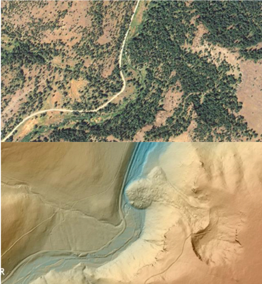
Figure 31. Baum and others (2014) showed that compared to other technologies, using 3DEP lidar data identified 3 to 200 times the number of landslides in densely forested areas.
